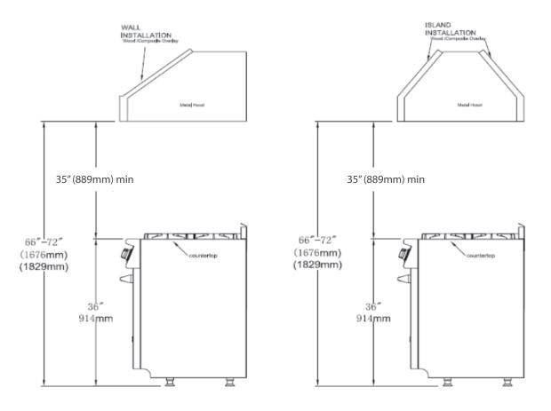
The bottom of the hood should be 35" min. to 36" above the counter top. This would typically result in the bottom of the hood being 66" to 72" above the floor. These dimensions provide safe and efficient operation of the hood.
